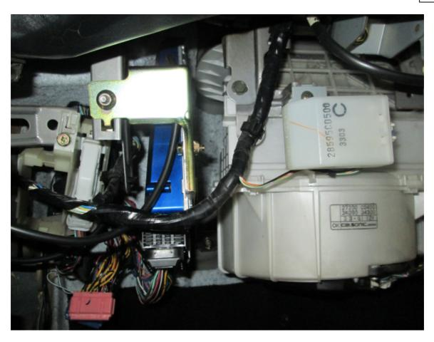
6. Install a vacuum line from the MAP port on the ECU to the intake manifold of the engine. The engine has a convenient port for connection under the front plastic engine cover.
