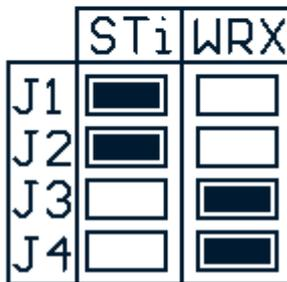
Depending on the country the vehicle was destined for the labelling of these jumpers (WRX and STi) may be incorrect. It may be necessary to try both options to determine which one is correct. If your vehicle is an STi and the ECU powers up with jumpers in the WRX position don't be alarmed.
