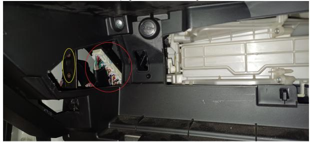
View of ECU Plugs from where the glovebox is located, note picture is from a RHD car.
