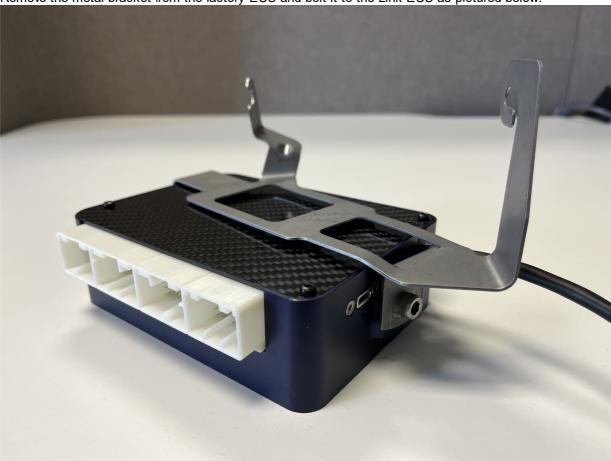
2. Remove the metal bracket from the factory ECU and bolt it to the Link ECU as pictured below.
