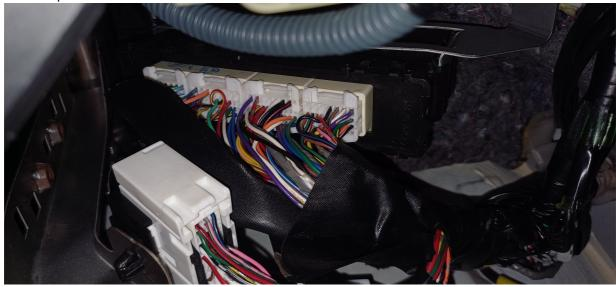
Picture of the Factory ECU from underneath the dash
