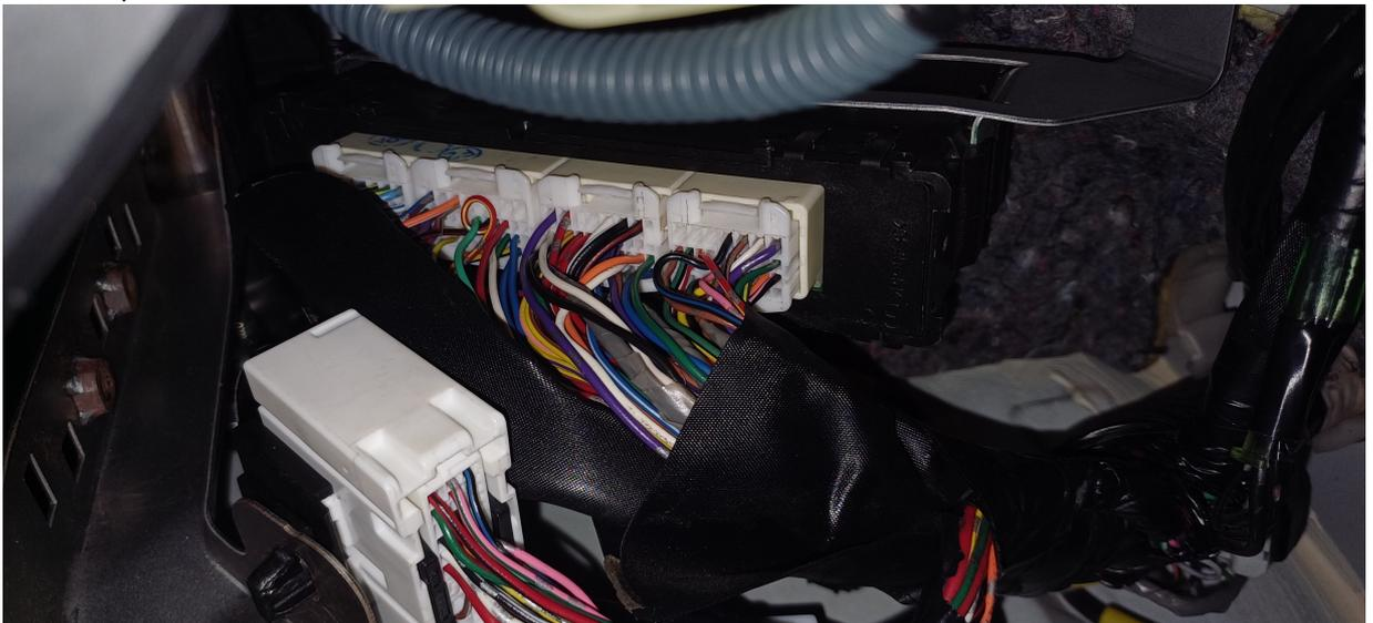
Picture of the Factory ECU from underneath the dash
