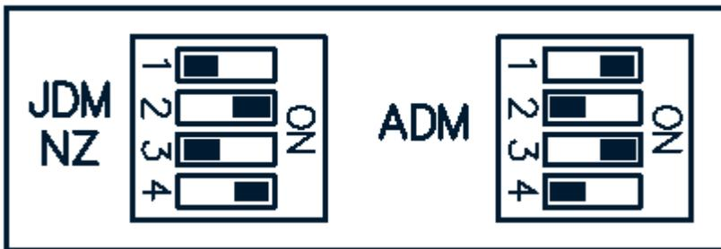
If your ECU bottom board is version 1.2 or higher, you will have a second set of jumpers. The jumpers are used to configure the board for either a 1991 - 1993 or a 1994 - 2002 SR20DET.
