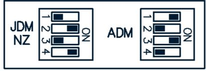
The jumpers are used to configure the board for either a 1991 - 1993 or a 1994 - 2002 SR20DET. Warning: Confirm the vehicles pinout against the information provided in the rear of this manual before configuring and installing the ECU.
