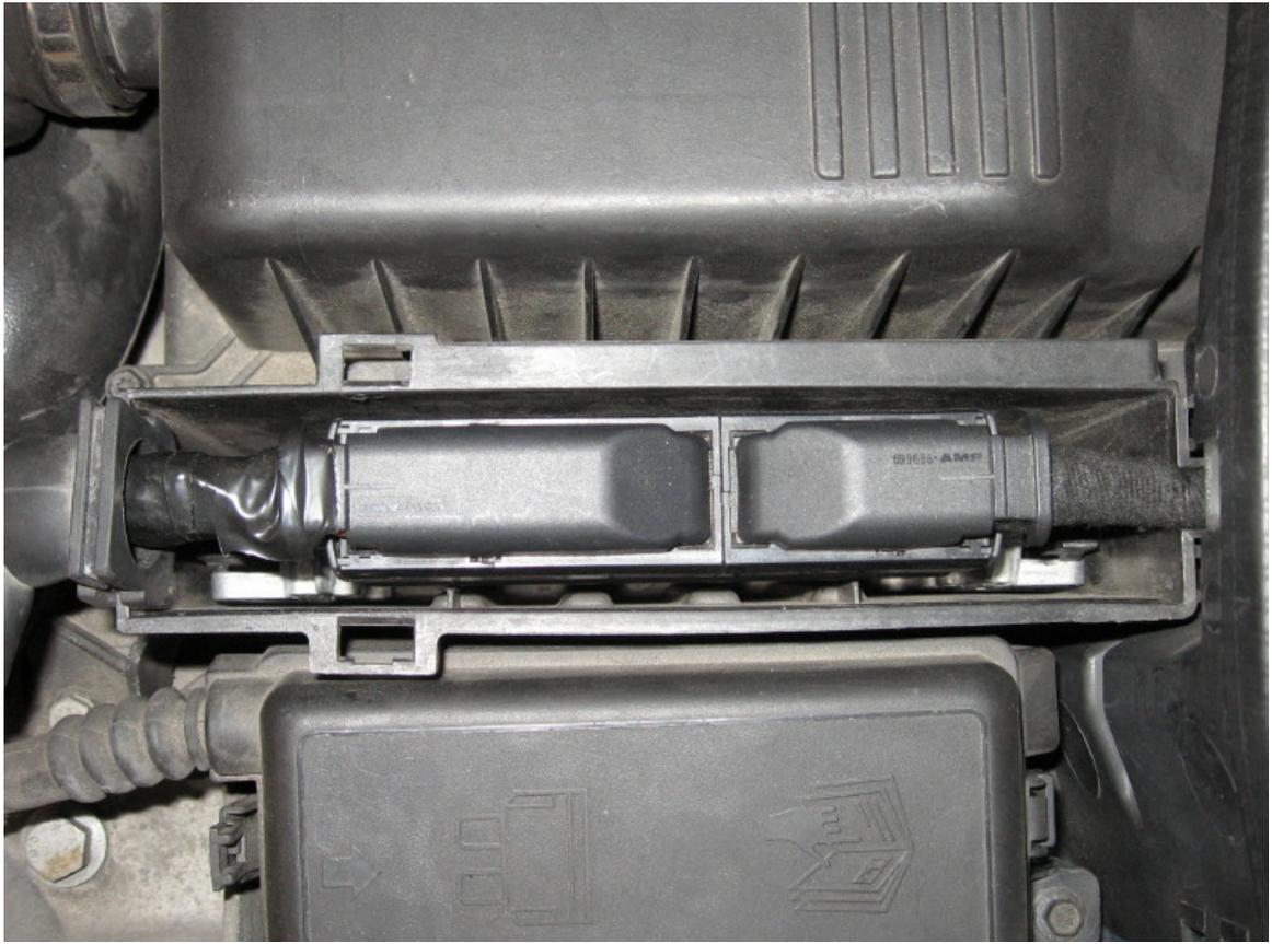
2. Install the Vi-PEC ECU into the factory ECU's position. Reinstall any fasteners.
