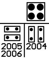
When the jumper consists of four pins in a square, correct selection is made by positioning the two jumpers in either vertical or horizontal orientation.
