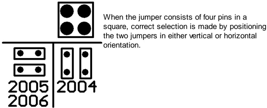
Information regarding the correct jumper position for the vehicle is printed on the PCB.
