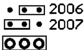
When the jumper consists of three pins in a row, correct selection is made by moving the jumper to the appropriate end of the three pins.
