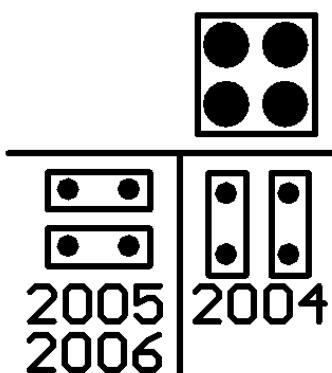
When the jumper consists of four pins in a square, correct selection is made by positioning the two jumpers in either vertical or horizontal orientation.
