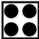
When the jumper consists of four pins in a square, correct selection is made by positioning the two jumpers in either vertical or horizontal orientation.
