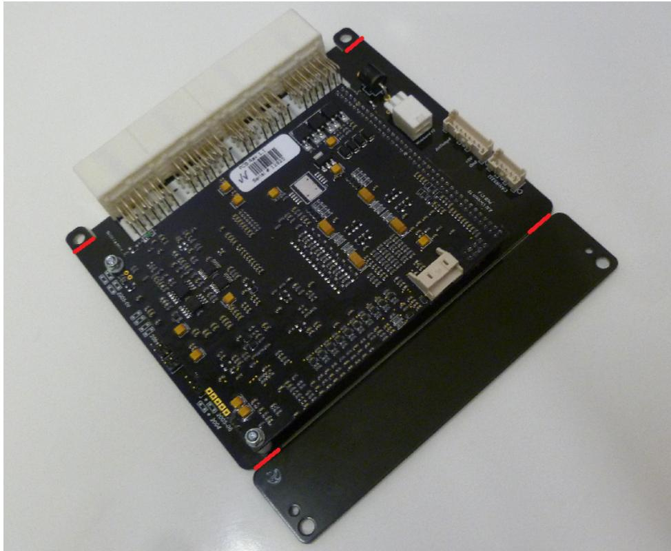
4. If the ECUs USB tuning cable is to be left permanently connected, a slot will need to be cut in the top cover. The best place to do this is usually beside the factory header.
