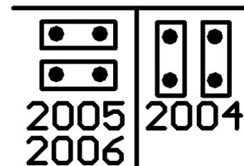
Information regarding the correct jumper position for the vehicle is printed on the PCB.
