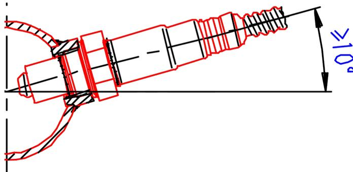
To avoid excessive heat the sensor should be mounted at least 1 meter from the engine exhaust port. Also ensure that the sensor is mounted greater than 1 meter away from the atmospheric end of the exhaust to ensure that readings are not contaminated by oxygen sucked up the exhaust. If the exhaust length is less than 2 meters then it is better to place the sensor closer to the engine.
